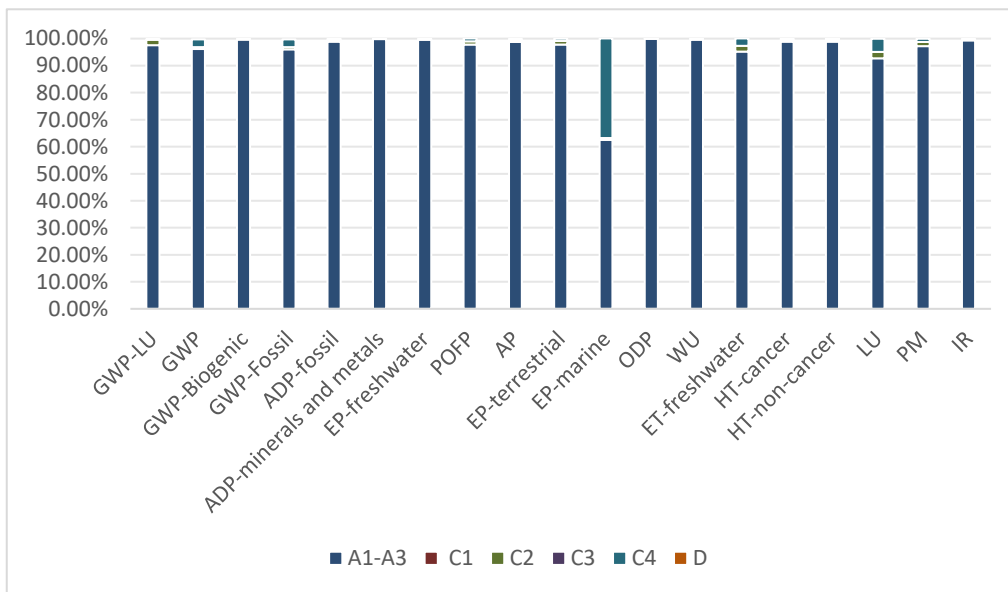
Figure 4. Creative Cut Screens each stage contribution to LCA results
