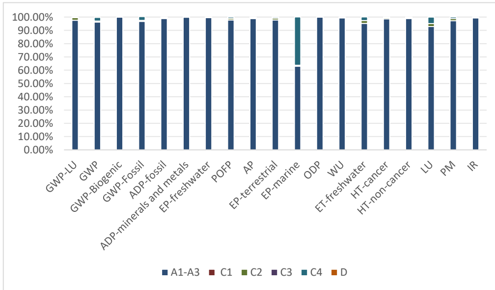
Figure 3. Layered Baffle each stage contribution to LCA results
